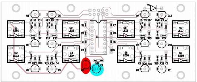
The front side of the board is mostly complete. Only the buttons and IC need to be installed. Before doing that, turn the board over and install the connector on the back.
